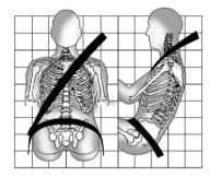
Sit up straight and always keep your feet on the floor in front of you. The lap part of the belt should be worn low and snug on the hips, just touching the thighs. In a crash, this
